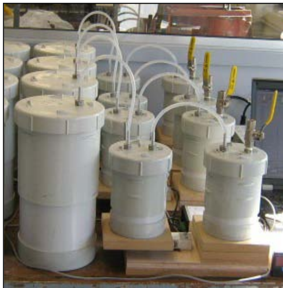
Plate 1: OxCon apparatus vessels including (from left to right) sample chamber, displacement chamber and fluid reservoir.
