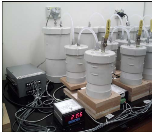
Plate 2: OxCon apparatus depicted with data logger, temperature transmitter and power supply.
