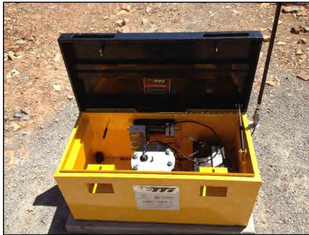
Plate 2: Gas monitoring instrumentation and enclosure typical of that at the Nevada and Sunny Corner mine sites.
